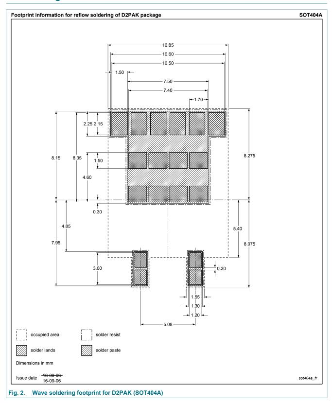
plastic, single-ended surface-mounted package (D2PAK); 3 leads; 2.54 mm pitch; 11 mm x 10 mm x 4.3 mm body
